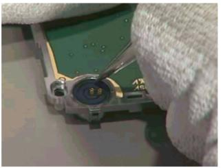
9. Remove the speaker by lifting it from the guiding pin.
