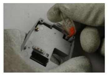
14. Remove the Vibra by lifting it out from its place
