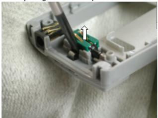
15. Remove the DC Jack by lifting it out from its place
