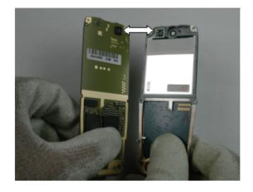
8. Remove the microphone by pressing it from its edge, or take the tweezers between the frame and microphone and lift it out from the frame.
