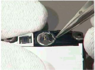
NOTE! The speaker is attached into the frame by adhesive tape. Therefore, it may not loose easily.
