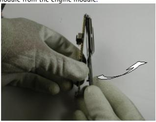
NOTE! The UI module and the engine board are linked together by two board-to-board connectors. Be careful not to damage them (see also next picture).
