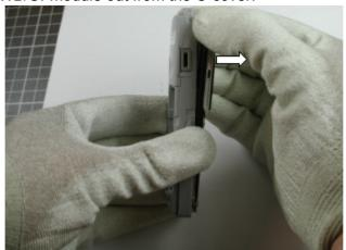
7. Remove the UI module from the engine module.
